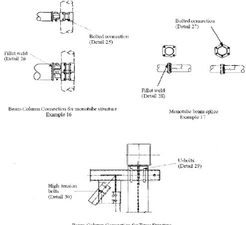
Beam-Cohunn Connection for Truss Structure Example 18
